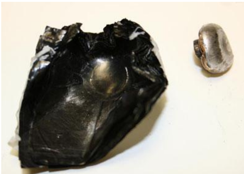
CNT fabric stopped a 9MM, jacketed round in controlled ballistics testing. This material shown is roughly the same thickness as six stacked business cards. (Source: Nanocomp Technologies)
