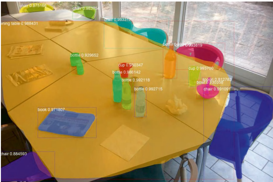
Figure 2-19. Example of a CNN detecting various objects on a table. Used with permission, source: https://www.ubiqisense.com/news/robot-to-clean-canteens [55]
