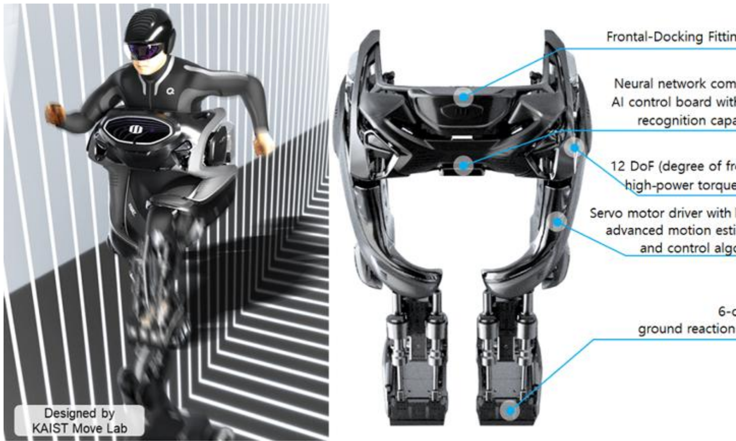
WalkON Suit F1 shape and main specifications. (CREDIT: KAIST)© The Brighter Side of News
