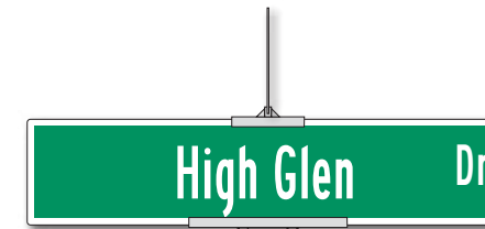
ST-Q.1 | Double Street Name w/ Stop 36"W x 8"H street; 24" STOP; 3" sq. alum. post QTY. 3 total
