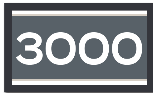
ST-F | Building Address 20"W x 12"H x 3MM ACM -surface printed graphics -brick wall mounted QTY. 19
