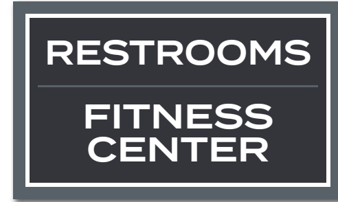
ST-7 | RR & Fitness Directional 20"W x 12"H x 3MM ACM -surface printed graphics -mounts to siding w/ undersized backer QTY. 1
