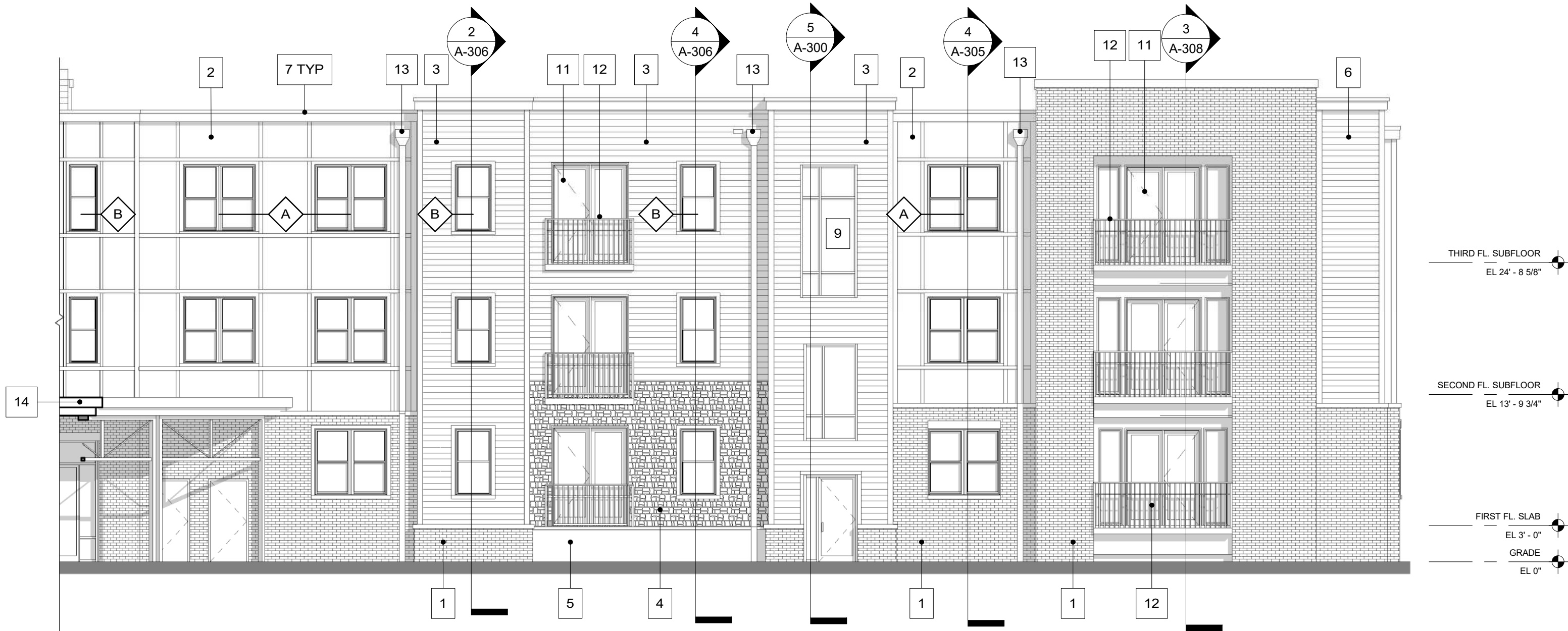
1 EXTERIOR ELEVATION - VIEW D 1/8" = 1'-0"
