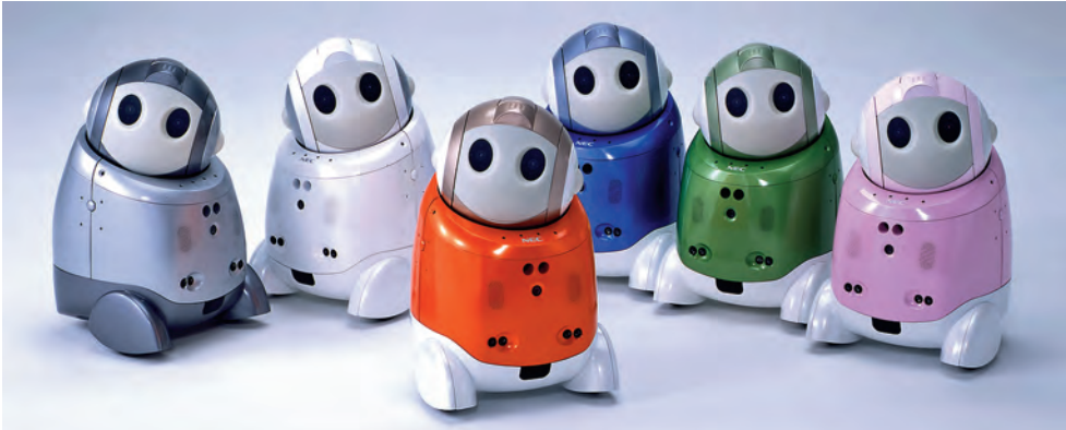
NEC's PaPeRo Personal Robot can respond to human voice and gestures and interacts wirelessly with other devices
