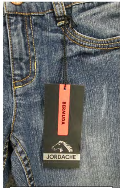
25-HT-33336159 BERMUDA HANGTAG PLACEMENT- WEARER'S FRONT LEFT BELTLOOP STRING IS LOOPED AROUND THE BELTLOOP 3" MAX CORD LENGTH
