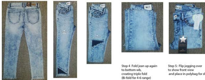
Step 1: Lay pant flat- facing back Step 2: Half fold jean at front rise vertical Step 3: Fold jean up to thigh area
