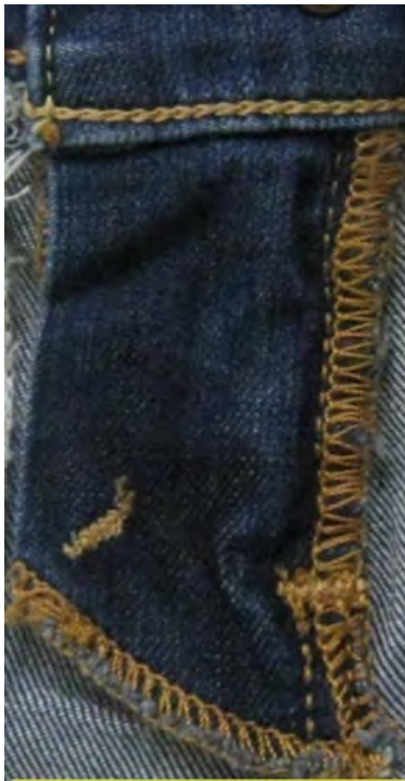
3 thread overlock bottom of front fly
