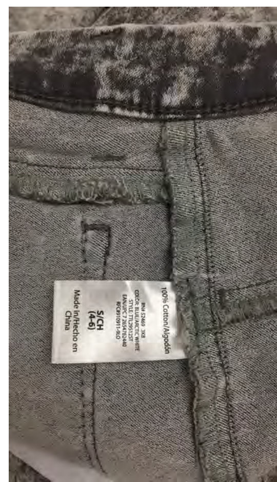
GENA 30048 GENERIC CARE LABEL PLACEMENT- WEARER'S LEFT, 2" BELOW INSIDE BOTTOM WAISTBAND, ON TOP OF THE STYLE LABEL
