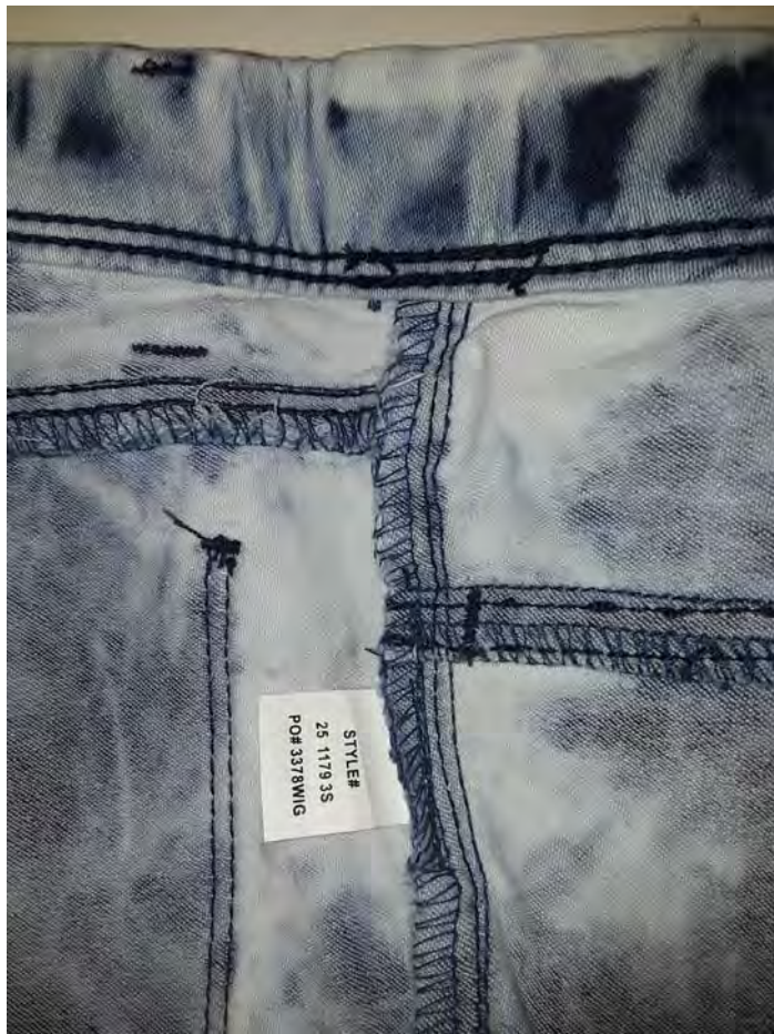
STYLE LABEL INSIDE WEARER'S LEFT SIDE SEAM 2" DOWN FROM BOTTOM WB, BEHIND CARE LABEL
