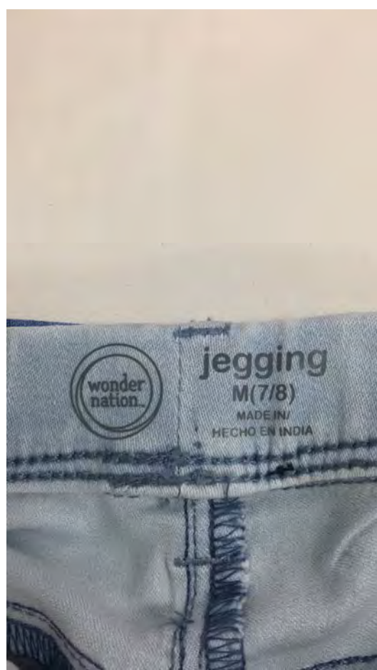
WNDM 37203 PLACED AT THE CB WAISTBAND SO THAT THE SEAM IS BETWEEN THE LOGO AND THE CALLOUT SECTION. THE HEAT SEAL SHOULD NOT BE PLACED ON TOP OF THE SEAM!
