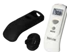
9306N Splash-Proof Dual Temp Infrared Thermometer with Fold Out Thermocouple Step Down Probe. HACCP pass/fail light system. Min/max/hold features. IP65 rated. Adjustable Emissivity. D:S=3.1. Thermocouple range: -67°/626°F and -55°/330°C. Infrared range: -67°/482°F and -55°/250°C. Thermocouple accuracy from 14° to 149°F (-10° to 65°C) +/-1°F (0.6°C). Infrared accuracy from 32°F to 149°F (0°C to 65°C). +/- 2°F (1°C). Resolution 0.5°F or 0.2°C. Auto shut off. Two AAA batteries included.
