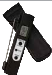
9305 Dual Temp Combination, Infrared and Thermocouple Thermometer. Min/max and hold features. CR2032 lithium battery included. Infrared temperature range: -27°F/428°F or -33°C/220°C. Probe range: -67°F/630°F or -55°C/330°C.
