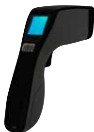
9305 Dual Temp Combination, Infrared and Thermocouple Thermometer. Min/max and hold features. CR2032 lithium battery included. Infrared temperature range: -27°F/428°F or -33°C/220°C. Probe range: -67°F/630°F or -55°C/330°C.
