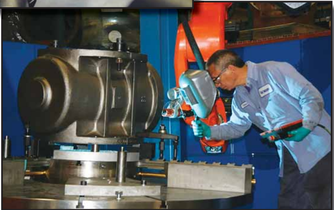
State-of-the-art robotic welding system for Cam-Centric® Plug Valve
