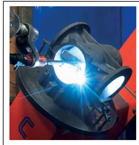
Figure 4. Robotic welding of nickel seat
