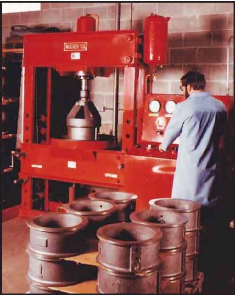
Dual Disc® Check Valve Hydrotesting
