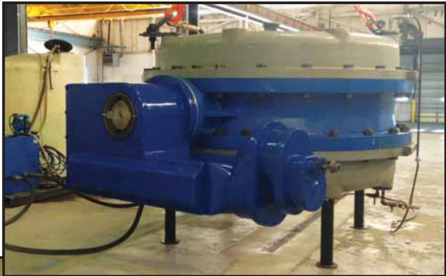
American-BFV® Butterfly Valve on Test Stand
