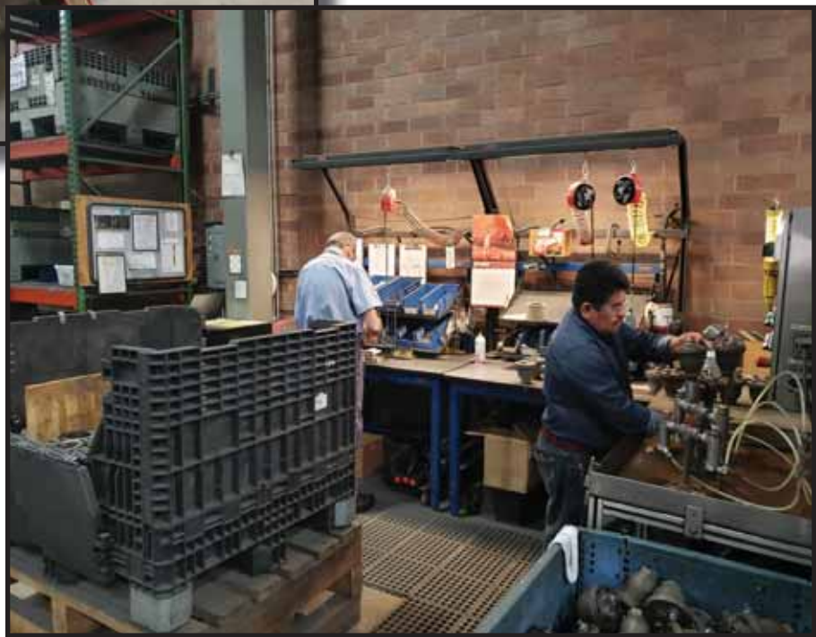
Air Valves are hand assembled and tested per AWWA Standards.
