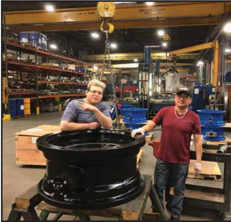
American-BFV® Butterfly Valve with Mechanical Joint Connections
