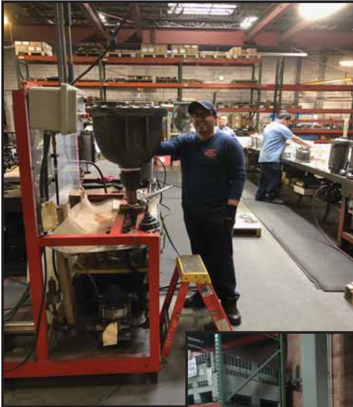
Air Valves are hand assembled and tested per AWWA Standards.
