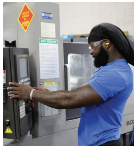
Clifton Graham, Machinist 1, operates the controls on the EMO 95, which produce seats for the trim sets.
