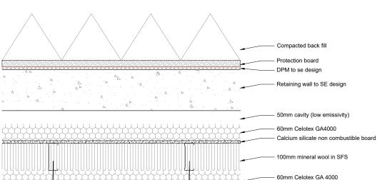
Joints taped and jointed to form VCL
