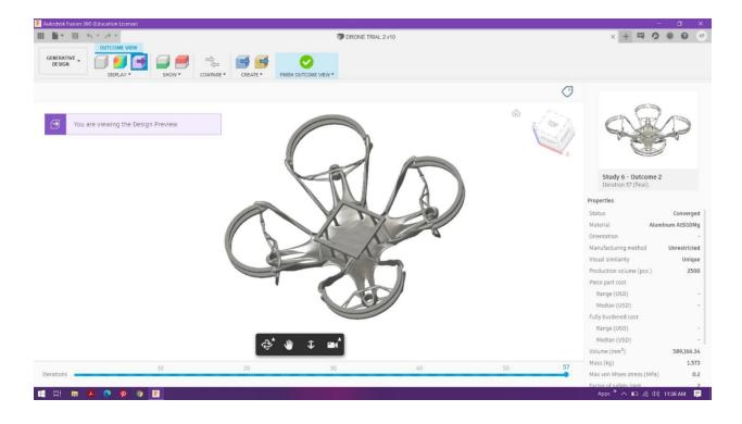
The above outcome was chosen at it satisfies both, the aesthetics and the function for the drone frame. The whole purpose of the drone frame is for the body to be light for aerial motion, for propellers to carry the body in upward movement.
