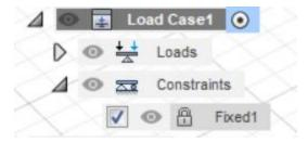
The Constraints put are fixed constraints on the drone propeller frame.
